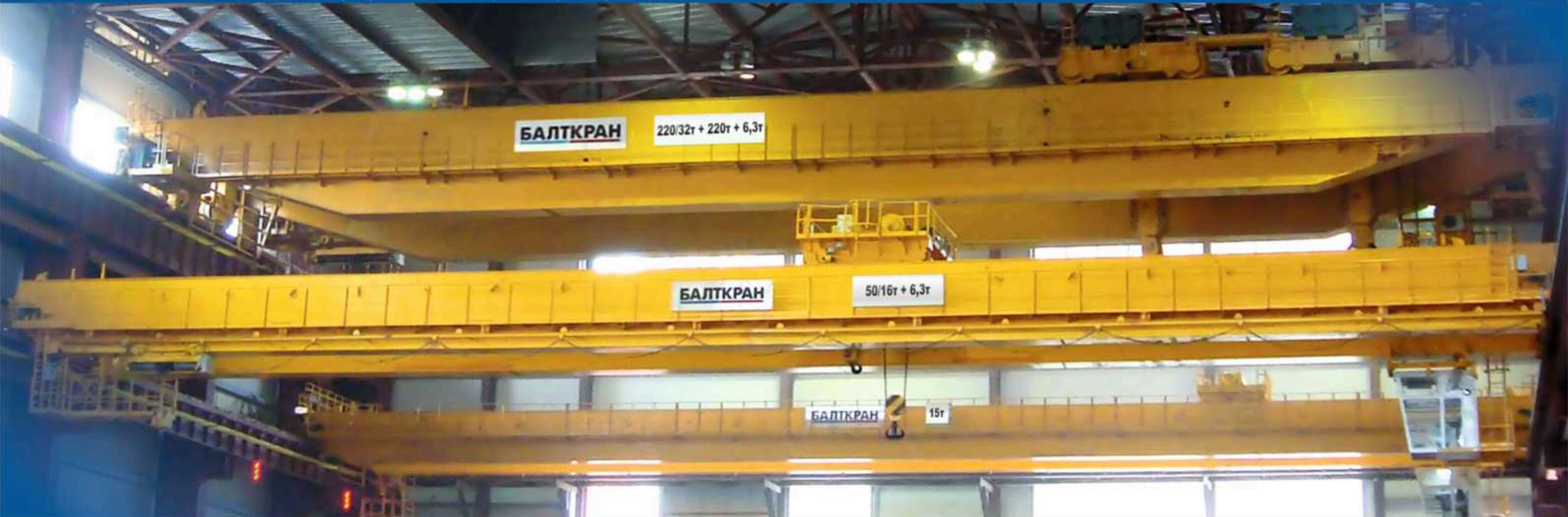
Novovoronezh nuclear power plant-2, turbine house, 3 cranes, L=45 m, anti collision system for cranes and loads.
